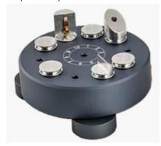
• Multi-angle preparation pods stand for horizontal, 45° and 90° pin stubs
